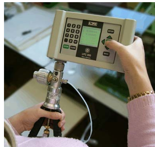
LPC 300 with calibration pump LPP 30 "on site"
