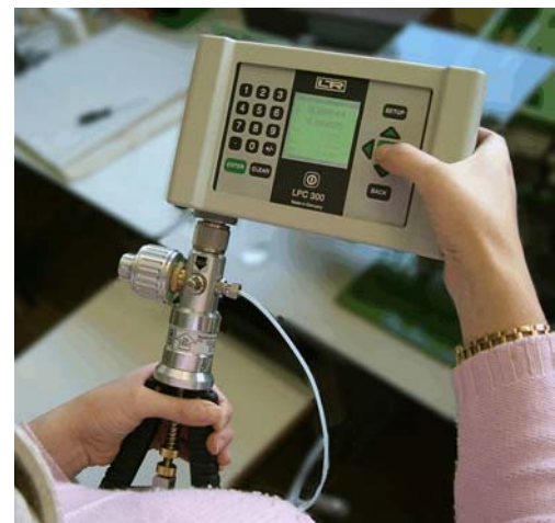
Calibration Test Pump LPP 30 with Electronic Calibrator LPC 300
