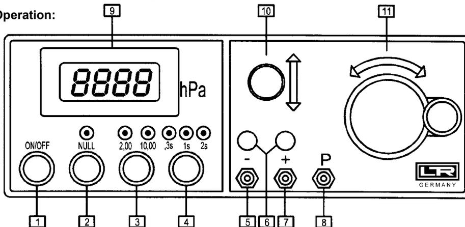
Pressure output P should be connected with 6 mm tube at a low or negative pressure using a T-piece to the pressure to be measured as well as to the pressure input "+" resp. "-" for vacuum. For large displacement volumes the measuring pressure is set to course using the pump [10]. Fine setting is made with knob [11].
